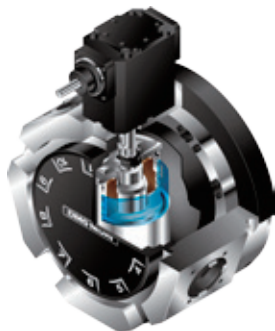
Milling turret designed to control thermal displacement (BMT)
